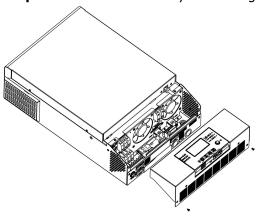
**Step 2:** Remove two screws as below chart and remove 2-pin and 14-pin cables. Take out the board under the communication board.
