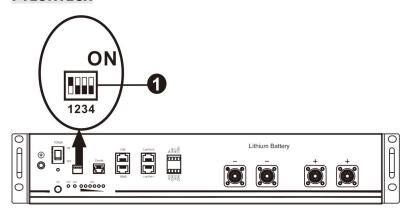
Dip Switch: There are 4 Dip Switches that sets different baud rate and battery group address. If switch position is turned to the "OFF" position, it means "0". If switch position is turned to the "ON" position, it means "1".
