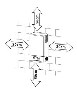
Install the unit by screwing three screws. It's recommended to use M4 or M5 screws.
