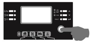
Step 5. Be sure to select battery type as "PYL" in LCD program 5.
