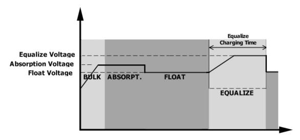
However, in Equalize Mode, if the battery equalization timer runs out and the battery voltage doesn't recover to the battery equalization voltage point, the charge controller will extend the battery equalized time until battery voltage achieves equalization voltage. If the battery voltage is still lower than equalization voltage when the extension runs out, the charge controller will stop equalization and return to the floating charging stage.
