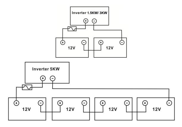
3. For the 1.5KW model, remove the insulation sleeve for about 18mm for positive and negative wires. Connect the two wires to the proper screw terminal on the unit. For 3KW/5KW models, apply ring terminals to your battery wires and secure it to the battery terminal block with the bolts properly tightened. Refer to battery cable size for torque value. Make sure polarity at both the battery and the inverter is correctly connected and ring terminals are secured to the battery terminals.
