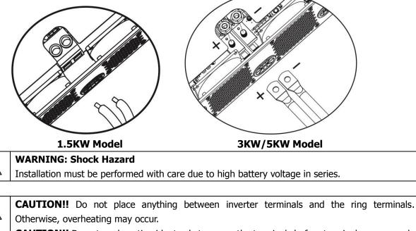
**CAUTION!!** Do not apply anti-oxidant substance on the terminals before terminals are securely tightened.
