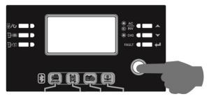
Step 4. Be sure to select battery type as "WEC" in LCD program 5.
