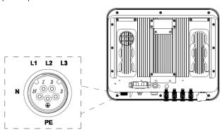
Fig 5.9 Three-phase inverter grid connection
