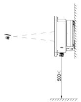
Fig4.3 Optimum installation height area
