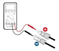
Fig 5.4 Measuring DC input voltage
