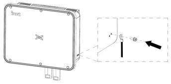
Fig 5.2 PV grounding diagram
