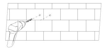
**Step 3:** Fix the hanging board. Clean the holes, use a rubber hammer to drive the expansion bolt into the hole, use a wrench to tighten the nut to fix the end of the bolt, then remove the nut, spring washer and flat washer, and then fix the wall mount plate to the wall and lock it with a tightening torque of  $13N^*m_\circ$ .
