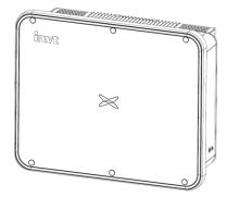
**Step 3:** After lifting the inverter, buckle the bracket plate on the back of the machine into the wall-mounting plate, and make sure that the machine bracket plate fits well with the groove of the hanging plate.
