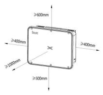
Fig 4.4 Installation spacing of inverter
