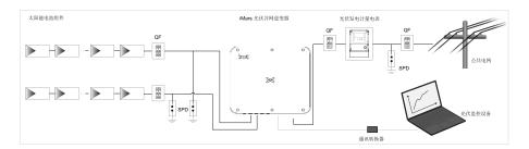
Fig 5.1 Schematic diagram of PV grid-connected system connection
