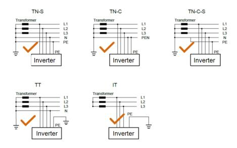
Fig 2.2 Grid forms supported by PV grid-tied inverters
