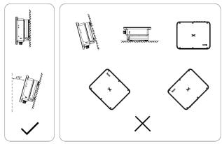
Fig 4.6 Installation position of inverter
