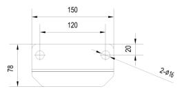
Fig 4.7 Dimensions of the mounting plate
