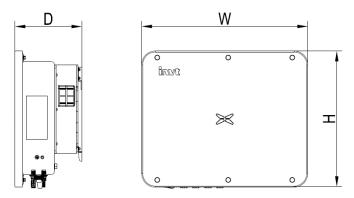
Figure 2.5 Outline dimensions of the inverter
